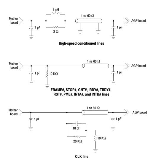
Figure 3-4: Equivalent circuit loads for the probe adapter
