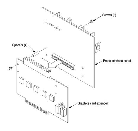
Figure 1-1: Connecting the probe adapter boards together
