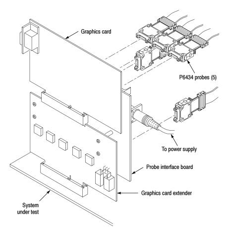
Figure 1-4: Connecting the probes to the probe adapter
