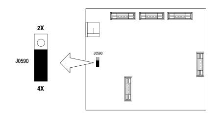
**12.** The data transfer rate (2X or 4X) must be selected using J0590 on the probe interface board. See Figure 1-5 for jumper location and settings.
