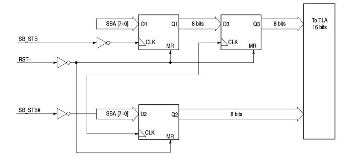
Figure 3-2: Block diagram for the SBA bus
