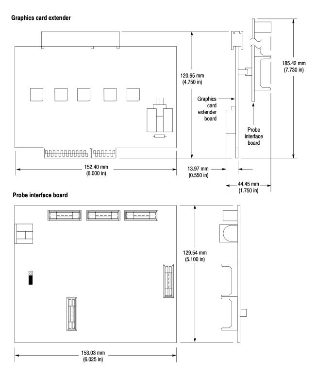
Figure 3-5: Probe adapter dimensions
