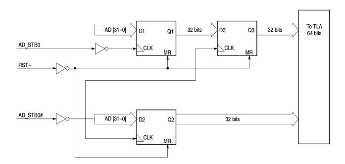
Figure 3-1: Block diagram for AD bus
