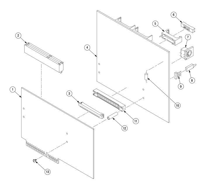
Figure 5-1: AGP4X probe adapter exploded view
