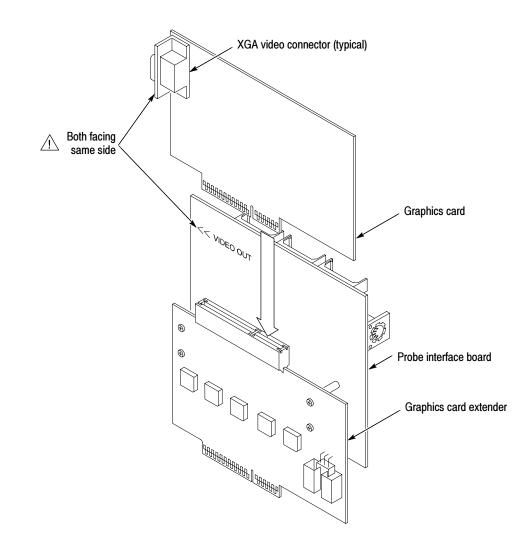
Figure 1-2: Connecting the graphics card to the probe adapter
